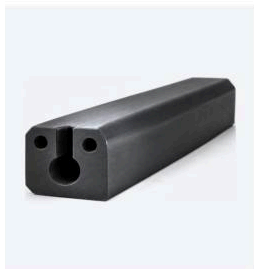
F.11 Key Hole Type Fender Keyhole bore with fixing holes for flush bolting to quays and pontoons.
